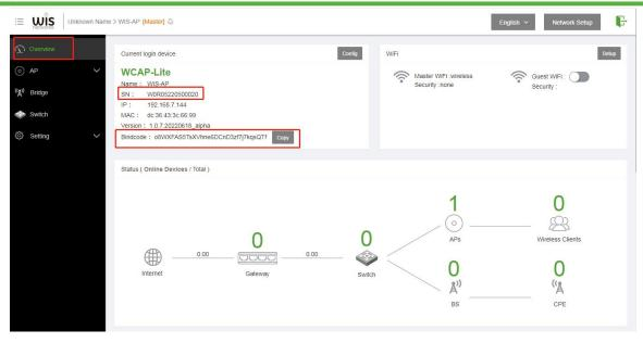
3.3 Click the device list to view the device information You can view the details of the device
